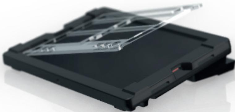
The keyguards are made from 5 mm thick plexiglass and can be supplied off-the-shelf or customized. They are milled instead of lasered to make sure the edges are **smooth and comfortable** for the user.
