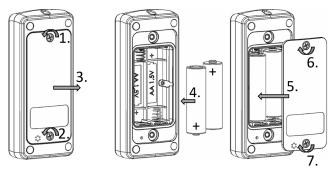
Always make sure that the seal of the battery lid is undamaged and free from debris before the lid is put back in place. Instruct the user on how to use the product in a safe way.
