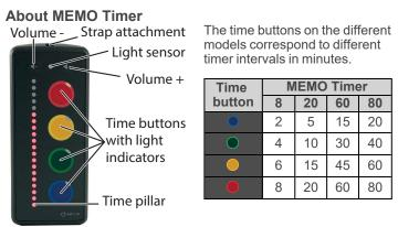
The light sensor adapts the brightness of the dots to the surrounding light. By using the provided straps, MEMO Timer can be carried around the neck or hung, for example, on a hook or in the shower.
