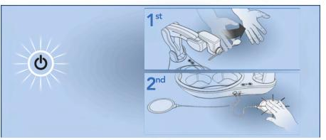
If the Power Button flashes, please remove the obstructing object. Once removed, touch either switch and the Arm will resume its motion.
