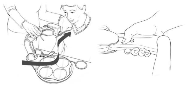
When the Teach Icon is covered, the Arm will be free for the Caregiver to move. The last two sections of the Arm will remain engaged and will keep the Spoon level when moving within the teach space. If resistance to movement is present, the thumb is probably not completely covering the Teach Icon.
